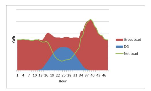
Figure 1: Diagram of Net Load Calculation
