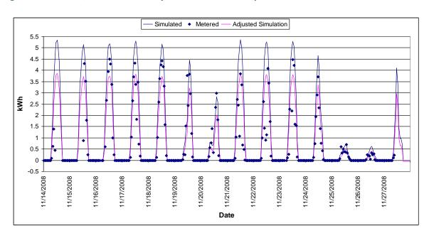
Figure 2: Simulated, Metered, and Adjusted Simulation Output Profiles of a PV Installation
