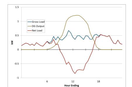
Figure 6: Load and DG Generation for an Example Residential Customer
