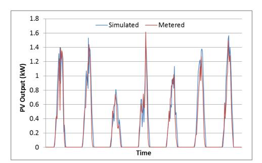
Figure 5: Simulated vs. Metered Solar PV for a Sample System During a Winter Week
