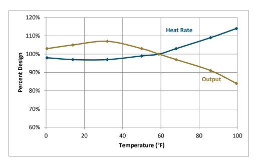
Figure 17: Temperature-Performance Curve for a GE LM6000 SPRINT Combustion Turbine
