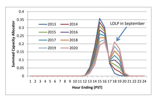
Figure 3: Capacity Allocator by Time of Day for the New Avoided Cost Methodology
