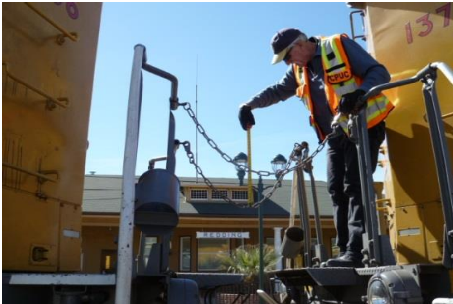
CPUC Operating Practices inspector measuring safety chain height
