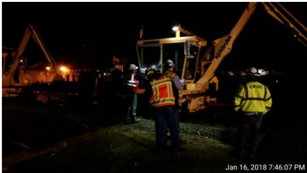
CPUC inspectors inspecting a tie crane at night during a focused inspection for operable change-of-direction alarm
