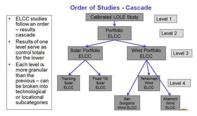
ELCC studies rely first on LOLE studies, and monthly ELCC studies require monthly LOLE studies. A Level 1 study is to calibrate the LOLE level of the overall electric system to the desired reliability level. Staff will add or remove electric capacity on a monthly basis in a predetermined order in order to result in a LOLE that is levelized and within the desired range, i.e. between 0.02 and 0.03.
