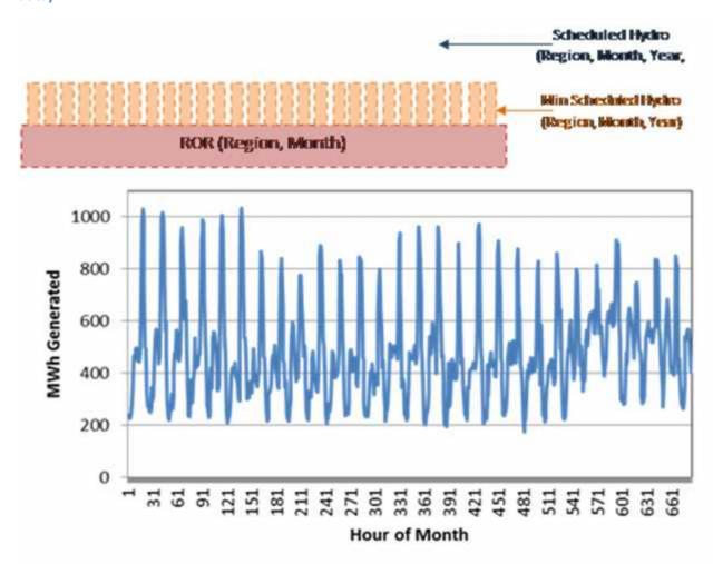
For facilities in Canada and Mexico, hydropower generation shapes are based on the closest neighboring US region (the Pacific Northwest and Arizona, respectively), and simply scaled to the region's maximum capacity.
