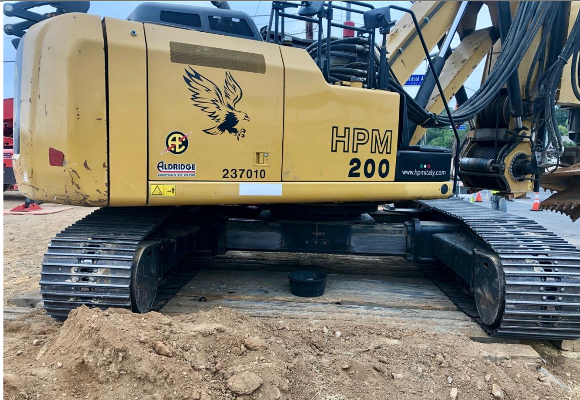
Photo 9 – The very small drip pan under the drilling rig.
