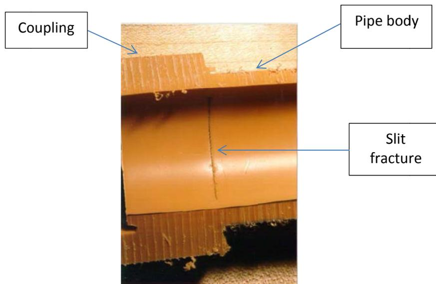
**Figure 1: Enlarged view showing slit fracture on the interior of 1 1/4 Inch Aldyl A service pipe involved in the San Juan incident**
