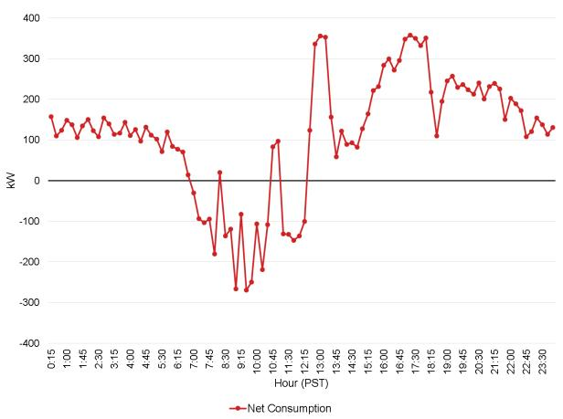
FIGURE 6-1: CUSTOMER 24-HOUR NET LOAD FOR OCTOBER 1ST
