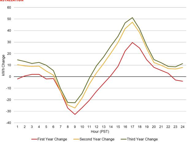
FIGURE 7-7: PG&E LARGE NON-RESIDENTIAL AVERAGE HOURLY CONSUMPTION CHANGES FOLLOWING PV INSTALLATION
