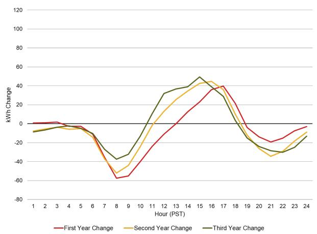
FIGURE 7-10: LARGE SCE NON-RESIDENTIAL CONSUMPTION CHANGES FOLLOWING PV INSTALLATION
