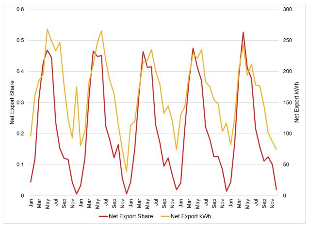
Figure 5-7 shows SDG&E residential net exporter share by month and systems size. The general shape is something between the other two utilities, with a peak in April (similar to SCE) and a larger share of systems net exporting in August (similar to PG&E). In April, 36 percent of systems under 3 kW and 77
