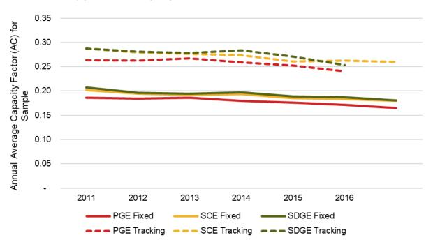
FIGURE 4-14: ESTIMATED AVERAGE ANNUAL CAPACITY FACTOR FOR ANNUAL IMPACTS SAMPLE BY ELECTRIC UTILITY AND ANALYSIS YEAR AND TRACKING TYPE\*
