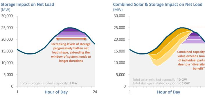
The ELCC approach inherently captures both **<u>capacity</u>** & <u>energy</u> adequacy
