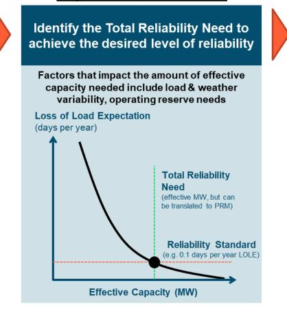
LOLP modeling provides Total Reliability Need in effective capacity MW to meet <0.1 days/yr LOLE, can be converted to a PRM
