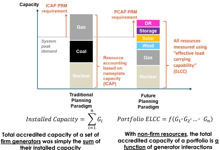
• Need determination: TRN/PRM defined based on Perfect Capacity (PCAP) MW
