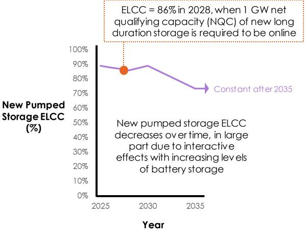
ELCC v alues from 2022 LSE plan filing requirements (38 MMT scenario) are used to define ELCC trajectory over time for new pumped storage
