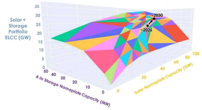
As RESOLVE adds solar and storage resources: (1) the portfolio ELCC increases and (2) the marginal solar and storage values may change if enough capacity is added to move to a different plane (each colored area is a plane)
