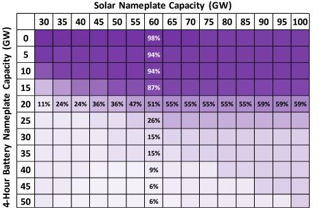
Battery marginal ELCC saturates without supporting solar capacity
