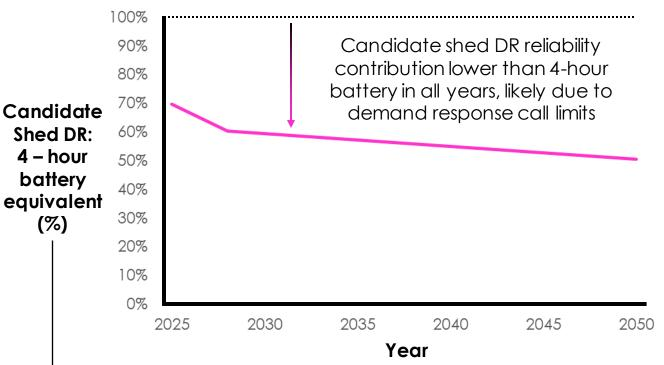
Y-axis represents candidate shed DR reliablity contribution relative to a 4-hour battery. 4-hour battery ELCC declines with increasing penetration via ELCC surface so candidate shed DR ELCC will also decline in the same manner
