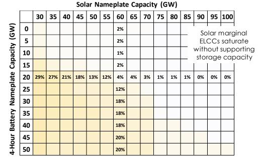
Batteries support solar marginal ELCC by shifting solar generation to hours when it is needed most
