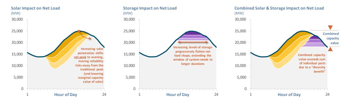
The ELCC approach inherently captures both **<u>capacity</u> & <u>energy</u>** adequacy
