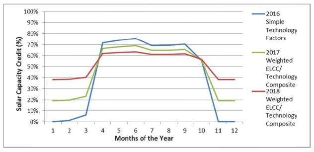
Figure 9 Proposed Phased in Composite Solar Monthly Factors versus 2016 Technology Factors
