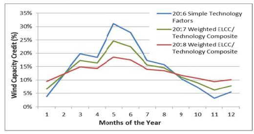
Figure 8 Proposed Phased in Composite Wind Monthly Factors versus 2016 Technology Factors
