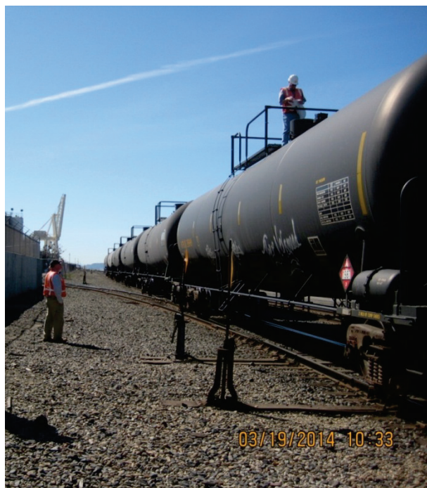
Hazmat tank car inspection, with CPUC Operating Practices personnel acting as lookouts
