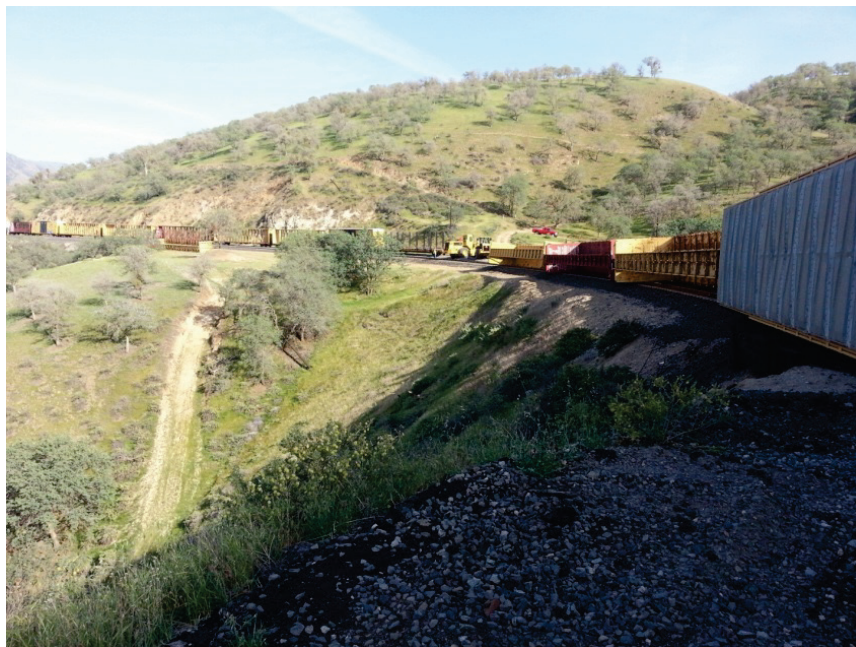
Derailed Cars – “String line” incident, near MP 342.75 at Cliff Union Pacific – Mojave Subdivision
