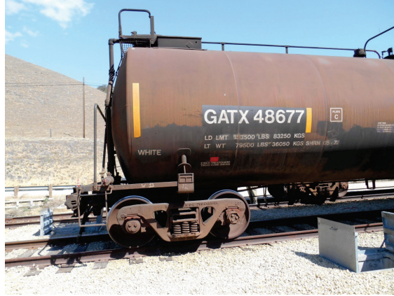
DOT 111-A Car built in 1977 travels between Central and Southern California as part of a unit train
