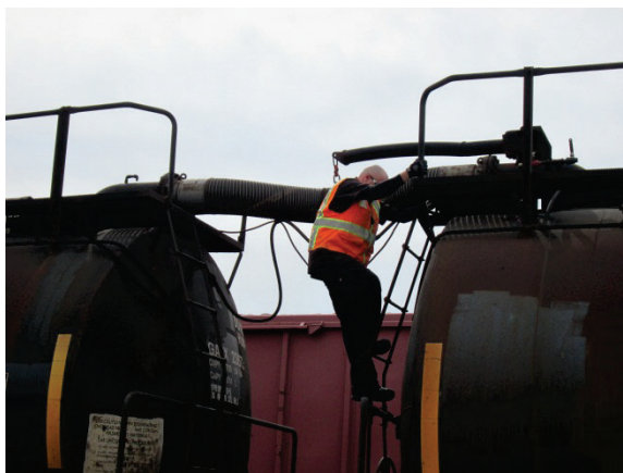
Inspecting typical DOT-111A tank cars on San Ardo to Dolores oil train. Some cars have a built date of 1977. Cars have a life expectancy of 50 years.
