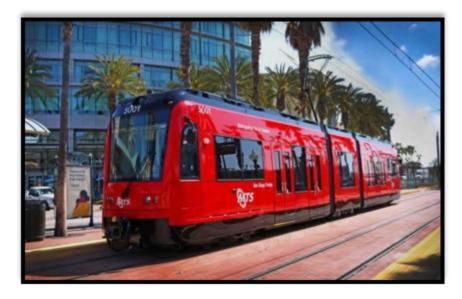
2020 with an expected schedule completion and acceptance of all 47 LRVs by late 2023. As Siemens cars are delivered on-site at the SDTI Yard, they will undergo commissioning and dynamics tests. Staff will participate in the acceptance testing throughout the procurement process and to date has accepted 14 LRVs for revenue service.
