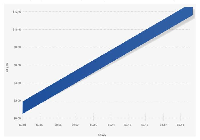
Image: EIN *Renewable Hydrogen Roadmap* 2018 Source data: ProtonOnsite - 2 MW PEM Electrolyzer at 2017 Costs
