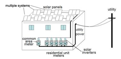
Figure 1: Conventional Solar Systems on Individually Metered Multifamily Housing
