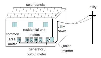
Figure 2: Virtual Net Metering System on Individually Metered Multifamily Housing
