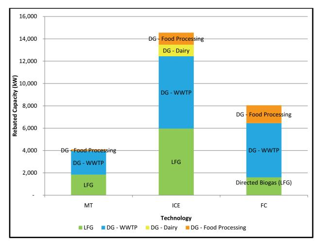
Figure 4: Contribution of Biogas Fuel Type by Prime Mover Technology
