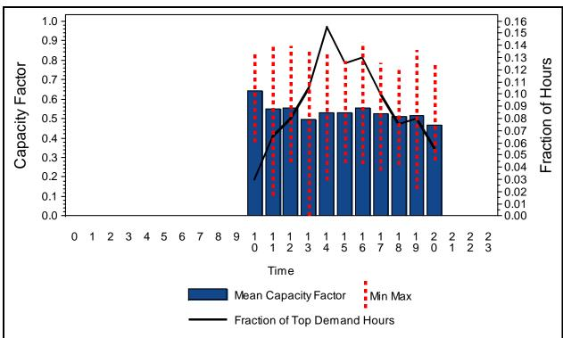
Figure A-11: DG Capacity Factor During Top 200 Hours of Feeder Demand on PG&E A
