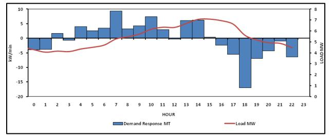
Since SCE provided hourly and not 15-minute data, the graph of the ramp rate is not as accurate as the PG&E feeder graph. The maximum rate of change for the 3.8 MW ICE unit is approximately 17 kW/min. A 17 kW/minute ramp rate is within the observed and rated ramping capabilities of an ICE unit The excess available power and the power from the ICE system is graphed in Figure 3-39.
