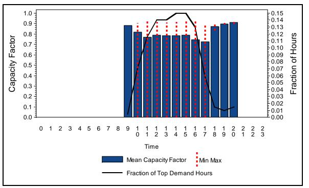
Figure 3-24: DG Generation during top 200 Hours of PG&E B Feeder Demand
