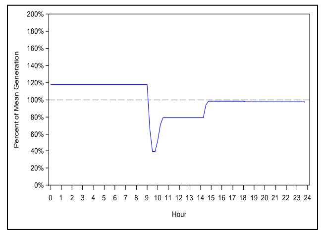
Figure B-2: Example of a Non-Volatile Load Day—Generation as Percent of Daily Mean
