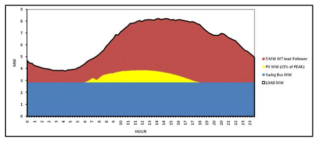
Figure 3-50: New Generation Profile with Fixed Swing Generation, Scaled PV, and MT Unit
