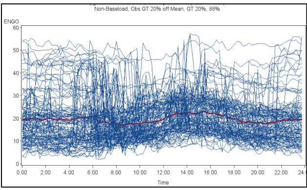
Figure 2-12: Non-Baseload Generation Profile for Process-Oriented Facility
