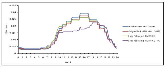
Due to the high line loading in this feeder, the average losses show a much smaller decrease than in previous analyses. The biggest decrease is the combination of ICE and PV, which removes the peak loss hours and decreases the MW losses by approximately 20%.
