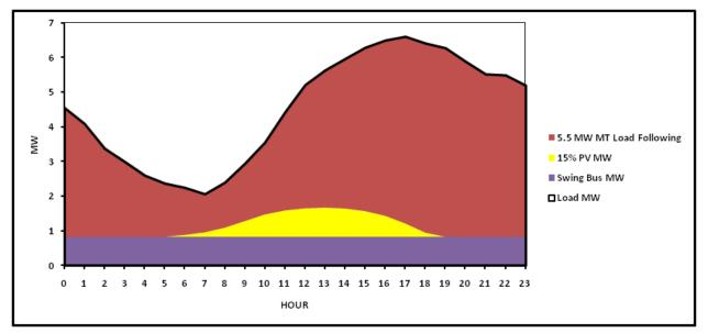
Figure A-28: SCE B DG MT Profile and Load Following Requirement
