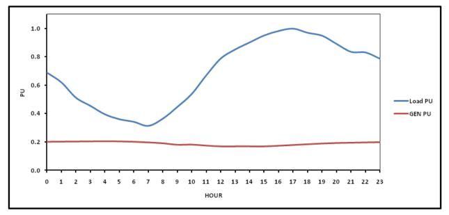
Figure A-26: SCE B Feeder Demand and 60 kW MT Profile
