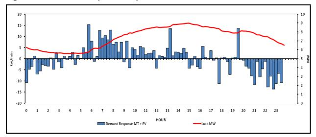
Figure 1-3: Demand Response Required for Microturbine Combined with PV
