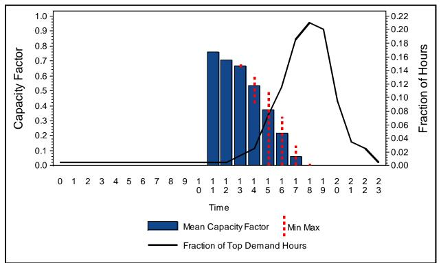
Figure A-21: DG Capacity Factor During the Top 200 Hours of Feeder Demand
