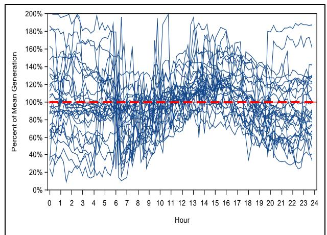
Figure B-3: Example of a Volatile Load, All June Days—Generation as Percent of Daily Mean
