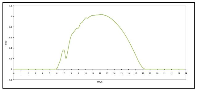
As shown in Figure 3-45, the SDG&E B feeder peak demand spans across much of the afternoon from 12 P.M. to 4 P.M.. In comparison, the PV generation peak of 114 kW occurs at 12:15 P.M.. There is a dip in the PV generation from 8 A.M. to 11:30 A.M. but the cause is unknown.
