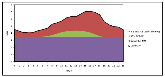
The ramp rate is calculated as previously described over each hour period (divided by 60 to give kW/minute). The resulting ramp rate requirement is shown in Figure 3-41. The maximum ramp down rate for the ICE unit is approximately 15 kW/min and the maximum ramp up rate is under 10 kW/min. A ramp rate of 15 kW/minute is within observed and rated abilities for an ICE unit.
