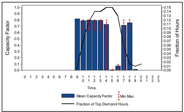
Figure A-3: DG Capacity Factor for Top 200 Hours of Demand on PG&E C
