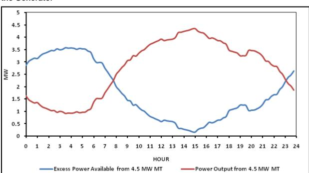
Figure 3-60: Call for Power for an Off-Peak Generator Plus Available Power from the Generator
