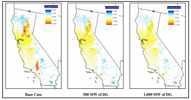
Table 3-12 provides a breakdown of the amount of installed DG capacity at each particular county associated with the top 200 WTLR values. The top 200 optimal bus locations are in PG&E and SDG&E only. Each of the counties has an associated climate zone. There is a total of approximately 310 MW of DG in PG&E's area and 190 MW of DG in SCE's area for a total of 500 MW of installed DG at the optimal locations identified by the power flow model.
