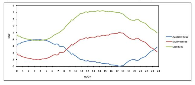
Figure 3-51: 5 MW Microturbine Generation and Excess Capacity
