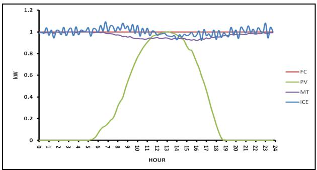
Figure 2-1: Typical DG Electricity Generation Profiles
