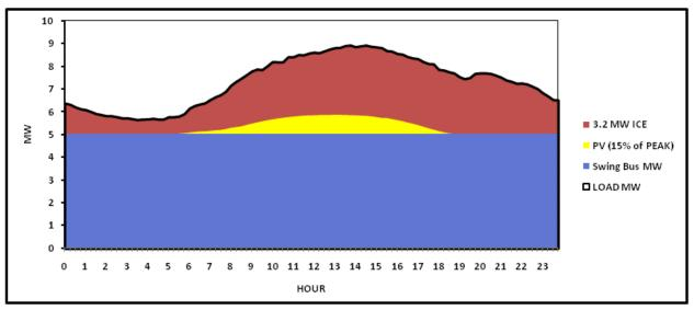
Figure A-4: Plot of PG&E C, Combined with 15% (1.3 MW), PV, and a 3.2 MW ICE
