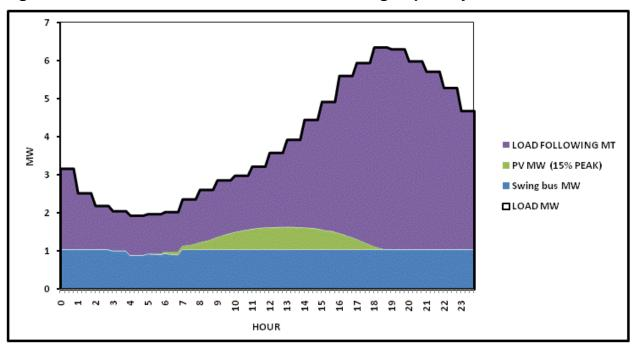
Figure A-23: New DG Profiles with Load Following Capability for SCE D
