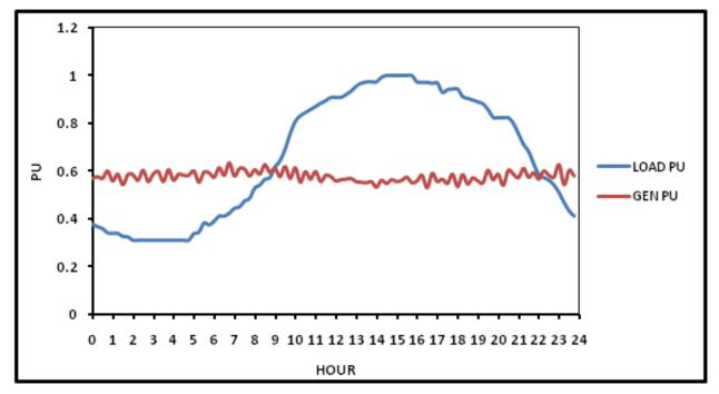
Figure A-10: Per Unit Load Profile and MT Generation Profile\*
