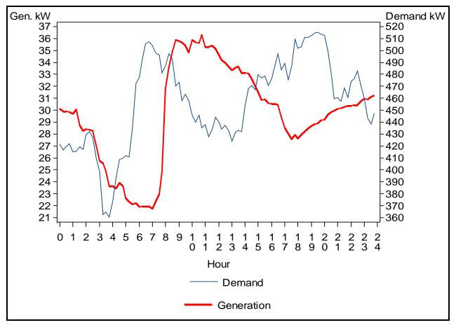
Figure 2-2: Characteristic Electrical Load Profile
