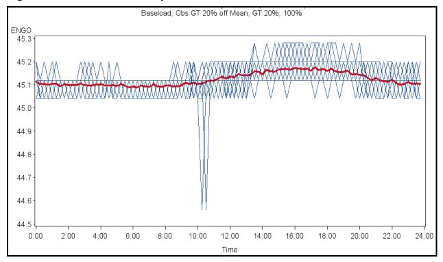
Figure 2-5: Condensed Hourly Generation Profile for a Fuel Cell
