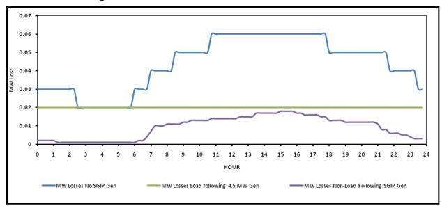
Figure 3-61: Losses are Minimized on the Feeder when Operating as a Non-Demand Following Generator
