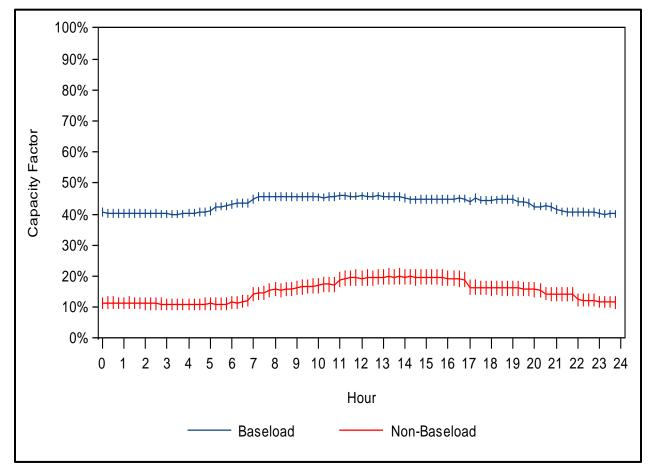
Figure B-6: Mean Generation Capacity Factors for Baseload and Non-Baseload, Inland
