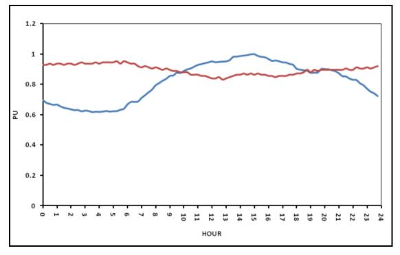
Figure 1-1: Example of Generator Output Against Demand
