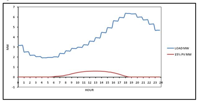
Figure A-20: SCE D Feeder Demand and 15% PV Profile
