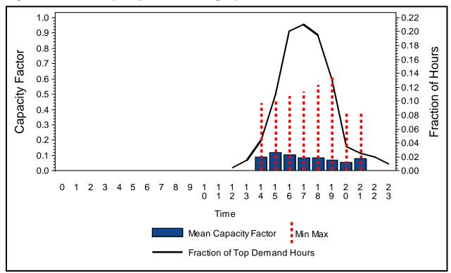
Figure A-27: DG Capacity Factor During top 200 Hours of Feeder Demand
