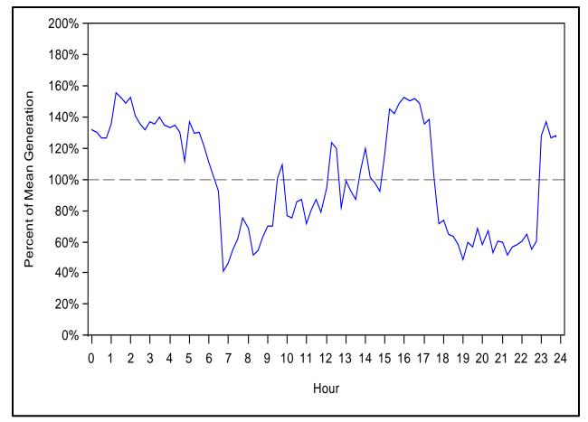
Figure B-1: Example of a Volatile Load Day—Generation as Percent of Daily Mean
