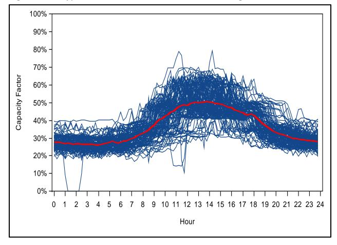
Figure B-11: Typical Non-Baseload Generation Profile, Single Peak
