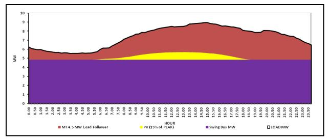
Figure 1-2: Dispatch of Swing Bus and DG Resources to Meet Feeder Peak Demand
