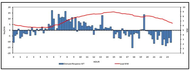
Figure 3-27: Ramping Required from the 4.5 MW MT Load Following System
