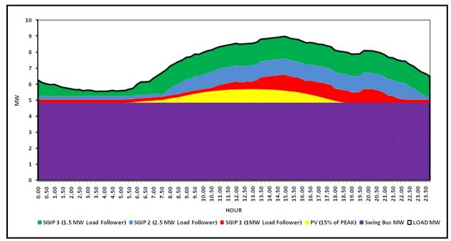
Figure 3-62: New Generation Blend for PG&E B
