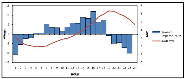
Figure A-24: Ramp Rate Required for New DG units on SCE D
