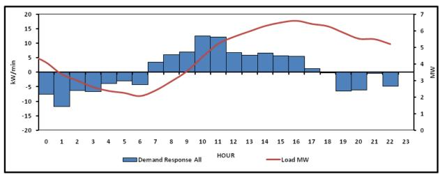
Figure A-29: Required Ramp Rate for Load Following Units on SCE B
