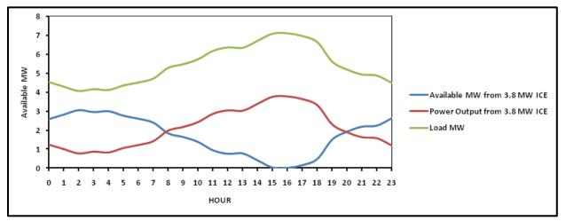
The DG unit dispatches and follows the load for the full 24 hours. At 4 P.M., it reaches maximum output. No excess power is available during the peak hour. The excess power from the ICE during off-peak hours also provides ramping capability.
