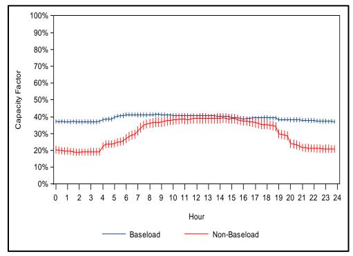
Figure 3-5: Average Capacity Factors for Baseload and Non-Baseload, Coastal
