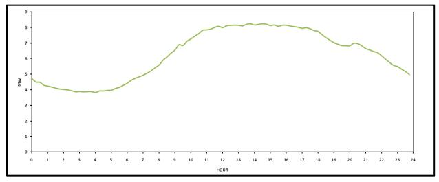
As with the previous feeder cases, SDG&E provided four months of data for the summer months from June to September 2008. No abnormalities were detected in the SDG&E B meter data. The generation profile of the PV units represent output of a typical PV generator, a bell curve with the peak energy production occurring in the afternoon hours. The generation profile is shown in Figure 3-46. The peak demand day occurred on August 7, 2008 and is the feeder profile used for this analysis.
