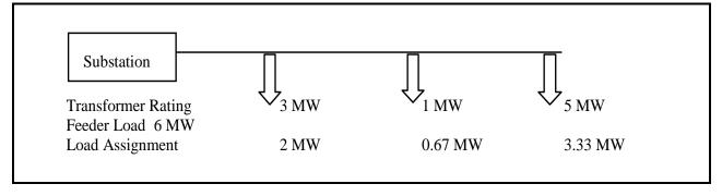
In this example, the total feeder load for this one hour is 6 MW but the total aggregated transformer capacity is 9 MW. The ratio of feeder load to transformer capacity is 0.67. Each transformer capacity is multiplied by the ratio to obtain the load assigned to each transformer. This prorating is required since the utility does not have the 15-minute loading on each individual transformer but only on the total feeder.
