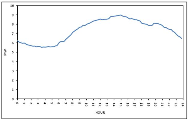
Figure 3-21: Demand Profile for Feeder PG&E B
