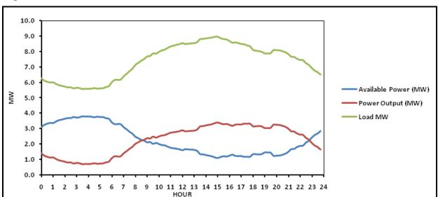
Figure 1-4: Available Power from the DG Generator Combined with PV
