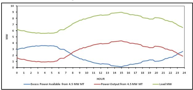
Figure 3-26: Output Power from the SGIP Generator with the Excess Power Available while Load Following
