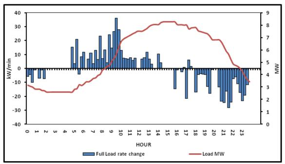
Figure A-13: Rate Required For 3 MW ICE Only
