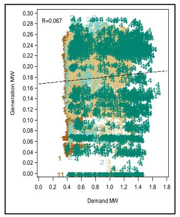
As an alternative illustration of the lack of relationship between generation and demand, Figure B-21 shows the mean hourly values for these variables. The percentage of total demand met by generation, which is annotated for odd hours, declines as the demand increases and the DG output remains fairly constant, which provides further evidence that the site represents a baseload profile.
