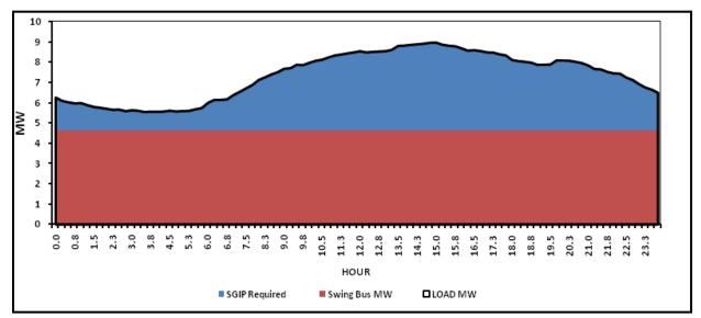
Figure 3-25: Demand Profile and the Contribution of Each Generator to the Profile
