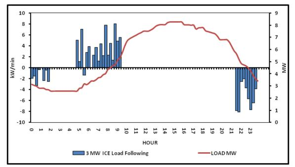
The available power from the scaled up ICE unit is limited during the maximum output hours as shown in Figure A-15. During the early morning minimum load period there is excess DG capacity, up to full capacity from 2 A.M. to 4 A.M.
