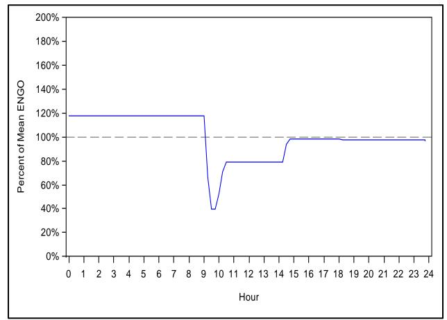
Figure 3-2: Example of a Non-Volatile Load Day—ENGO as Percent of Average ENGO
