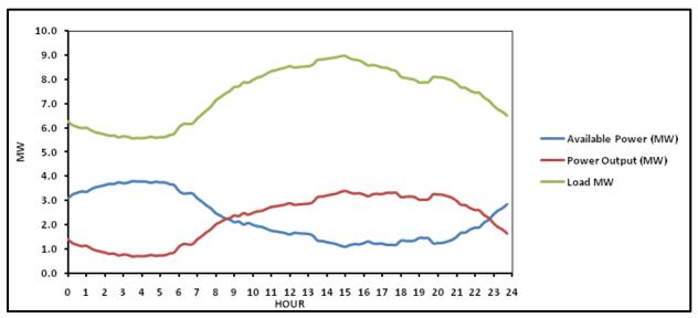
Figure 3-30: Available Power from the DG Generator Combined with PV
