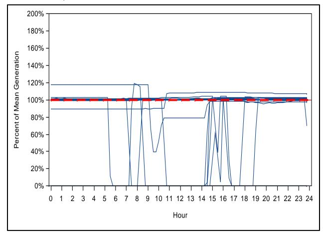
Figure B-4: Example of a Non-Volatile Load, All June Days—Generation as Percent of Daily Mean
