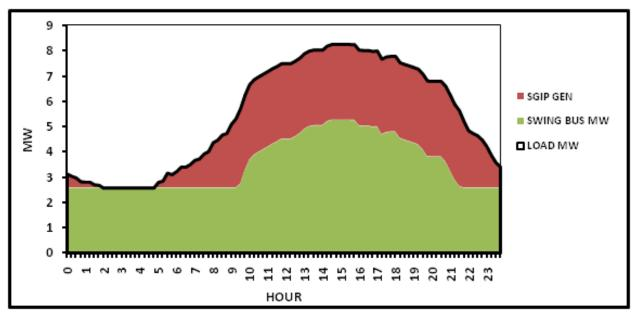
Figure A-12: Additional 3 MW ICE Unit Added To PG&E A's Generation Profile
