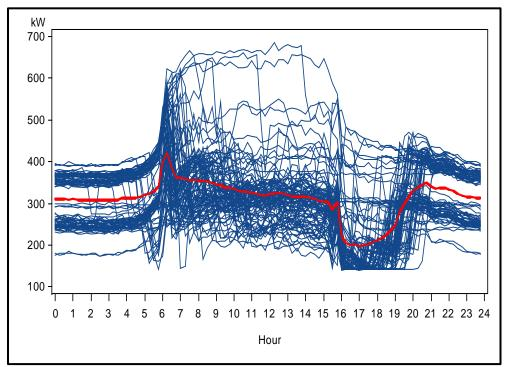
Figure 3-9: Plot of Metered Demand, All Days with Mean
