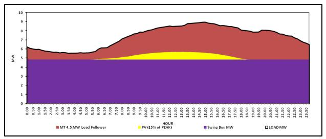
Figure 3-28: New Demand Profile with High PV Penetration Dispersed Across the Loaded Buses
