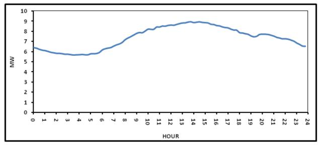
Minimum load is 5.67 MW at 4 A.M.; maximum load is 8.95 at approximately 2 P.M.
