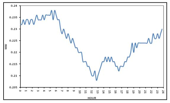
Figure 3-22: Generation Profile for SGIP Generator on PG&E B (250 kW MT)
