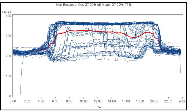
Figure 2-11: Non-Baseload Generation Profile for Occupancy-Oriented Facility
