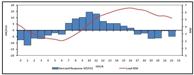
In Table A-7, the daily energy calculations are broken down by technologies and groups. If SCE B were provided with utility energy, the feeder would consume 108.6 MWh. However, with one 5.8 MW MT SGIP generator providing 87 MWh throughout the 24 hr period, the energy the swing bus will have to provide is 21.6 MWh. When the DG penetration was additional PV, the utility would provide 19.9 MWh, where as the MT provides 82.1 MWh and the PV unit contributing 6.7 MWh.
