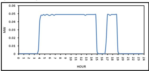
Figure A-2: ICE Original DG Load Profile
