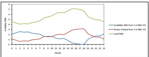
Figure 3-42: Available Power Plot from ICE and PV on SCE C
