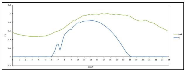
Figure 3-47: Per Unit Representation of PV and Feeder Demand for SGD&E B
