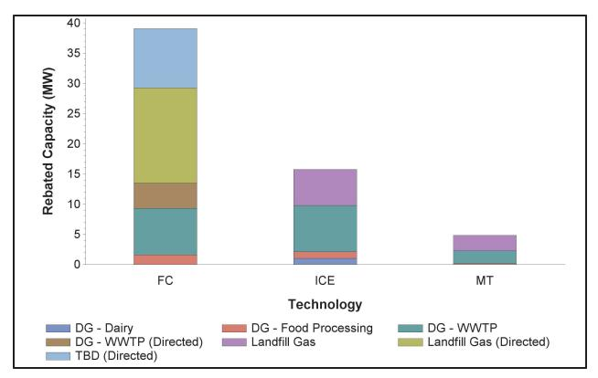
Figure 5: Contribution of Biogas Fuel Type by Prime Mover Technology
