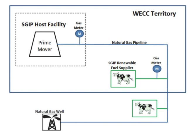
Figure 1: Schematic Depiction of Directed Biogas Arrangement
