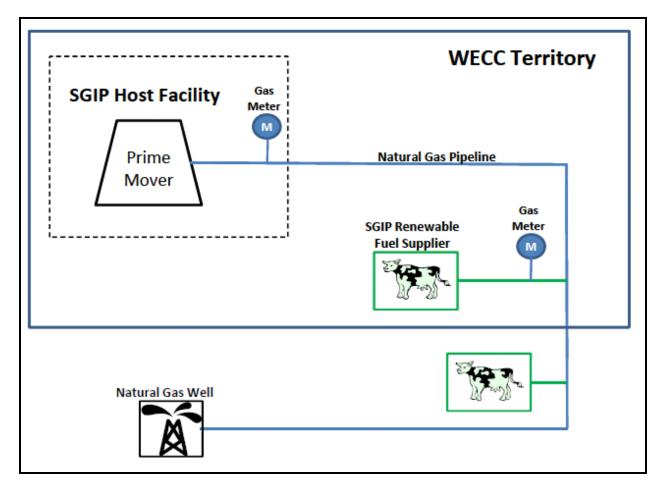
Figure 1: Schematic Depiction of Directed Biogas Arrangement
