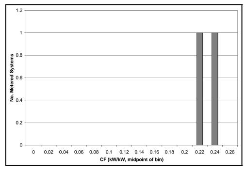
Figure D-39: PV (Tracking) Measured Energy Production (Capacity Factor)
