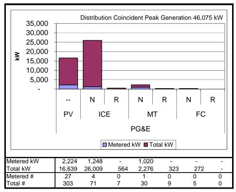
Figure B-17: Metered and Estimated Total Generation – PG&E
