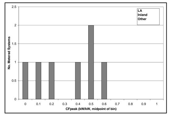
Figure D-17: LA (SCE & SCG) PV Measured Coincident Peak Output (Inland, Other)
