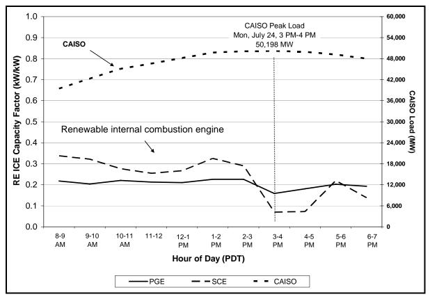
Figure A-23: CAISO Peak Day Capacity Factors by PA—ICE
