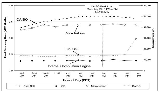
Figure 5-20: Heat Recovery Rate during CAISO Peak Day
