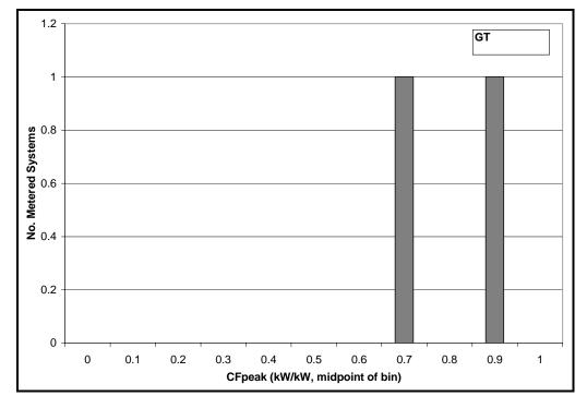
Figure D-31: Gas Turbine Measured Coincident Peak Output (Nonrenewable Fuel)
