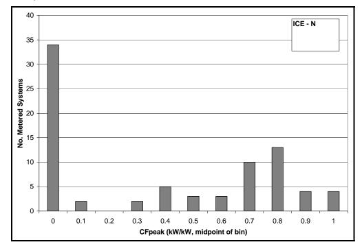
Figure D-27: IC Engine Measured Coincident Peak Output (Nonrenewable Fuel)
