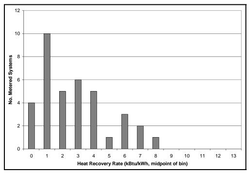
Figure D-51: Engine/Turbine Measured Heat Recovery Rate
