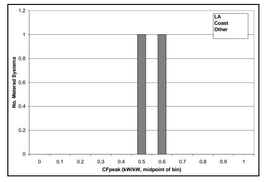
Figure D-13: LA (SCE & SCG) PV Measured Coincident Peak Output (Coastal, Other)
