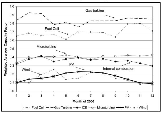
Figure A-5: Monthly Capacity Factors by Technology
