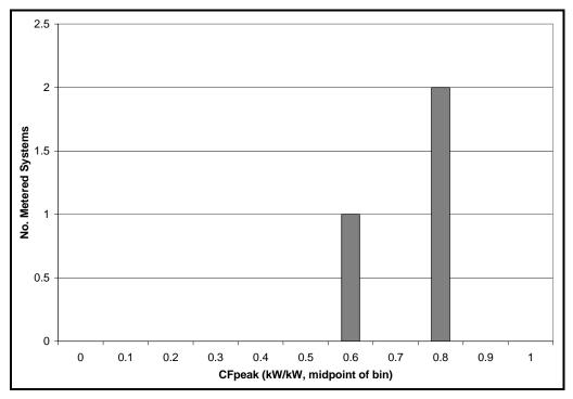
Figure D-9: PG&E PV Measured Coincident Peak Output (Tracking)
