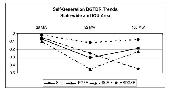
Figure 5-19: Results of DGTBR Impacts under Different Penetration Cases
