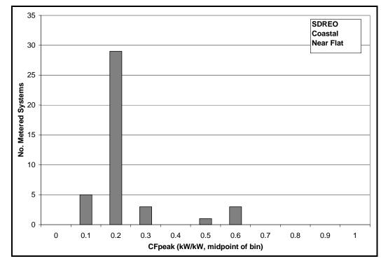
Figure D-21: SDREO PV Measured Coincident Peak Output (Coastal, Near Flat)
