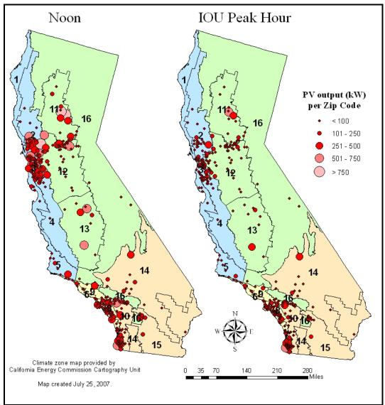
Figure 1-6: Impact of Peak Demand Time of Day on PV Capacity\*
