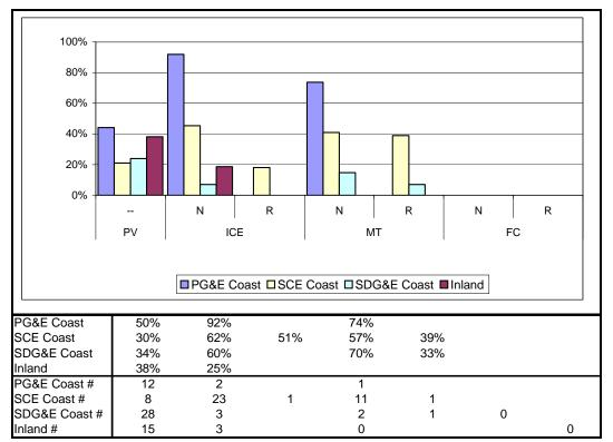
Figure B-25: Percentage of Capacity Operational By Climate Zone - 2006
