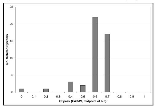
Figure D-1: PG&E PV Measured Coincident Peak Output (Coastal, Near Flat)
