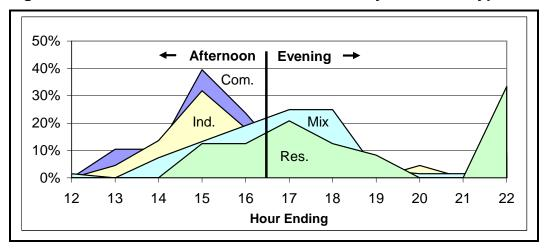
Figure B-11: Distribution of Feeder Peak Hour by Customer Types Served
