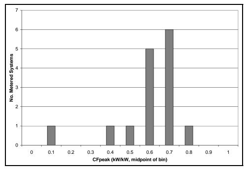
Figure D-3: PG&E PV Measured Coincident Peak Output (Coastal, Other)
