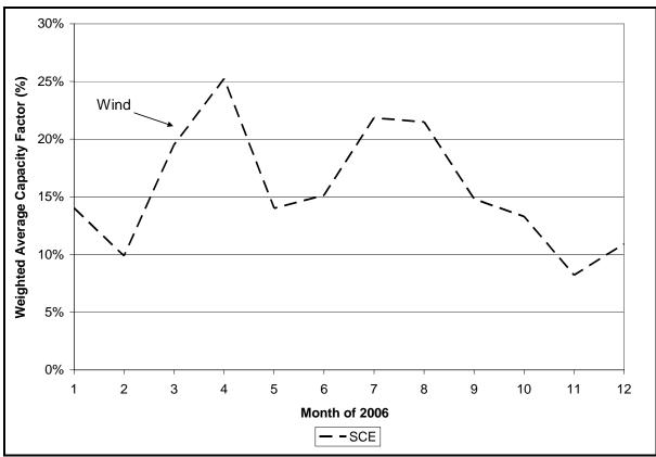
Figure A-15: Monthly Capacity Factors by PA
