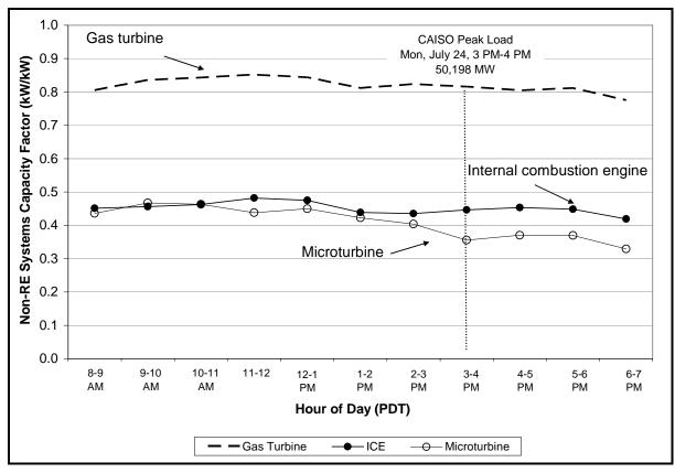
Figure A-35: CAISO Peak Day Capacity Factors by Technology
