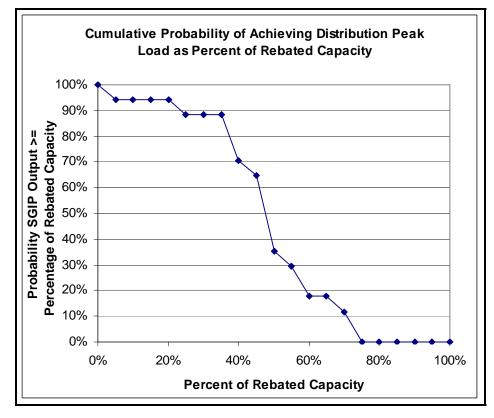
Figure 1-8: Probability of PV Output at Distribution Peak Hour (SCE Coast, Feeder Peak > HE 16)
