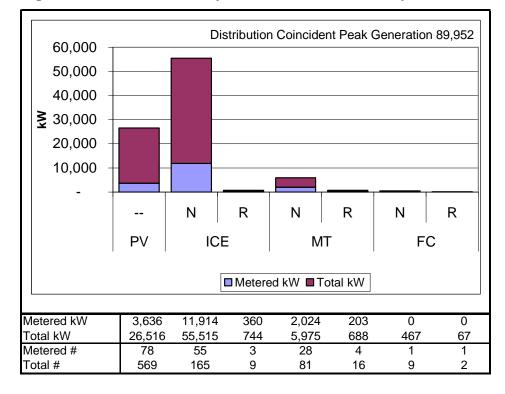
Figure 1-7: Distribution System Peak Reduction by SGIP Technology (2006)
