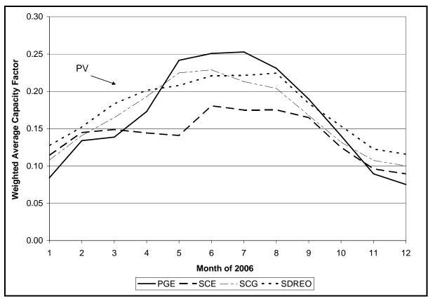
Figure A-10: Monthly Capacity Factors by PA
