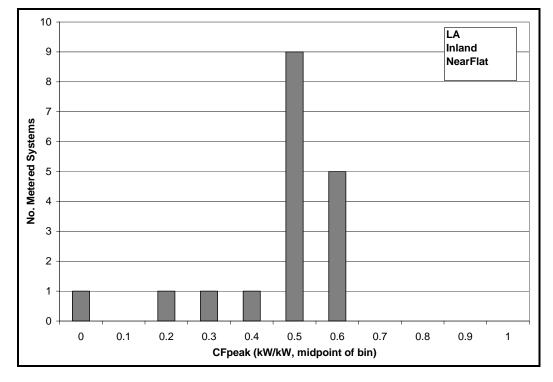
Figure D-15: LA (SCE & SCG) PV Measured Coincident Peak Output (Inland, Near Flat)
