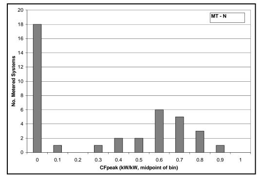
Figure D-33: Microturbine Measured Coincident Peak Output (Nonrenewable Fuel)
