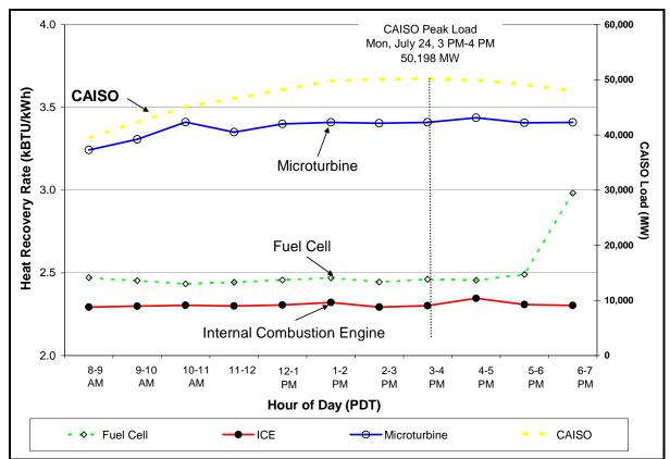
Figure 1-11: Heat Recovery Rate During CAISO Peak Day
