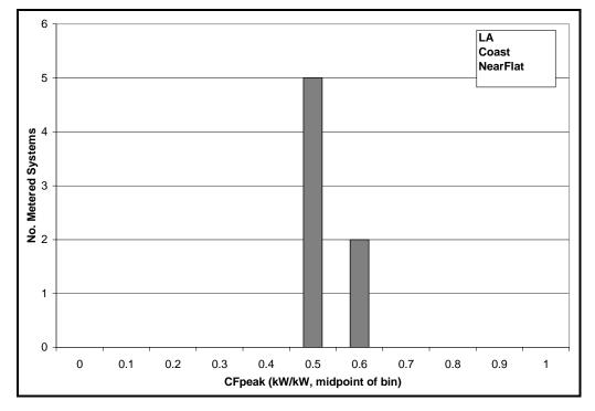
Figure D-11: LA (SCE & SCG) PV Measured Coincident Peak Output (Coastal, Near Flat)
