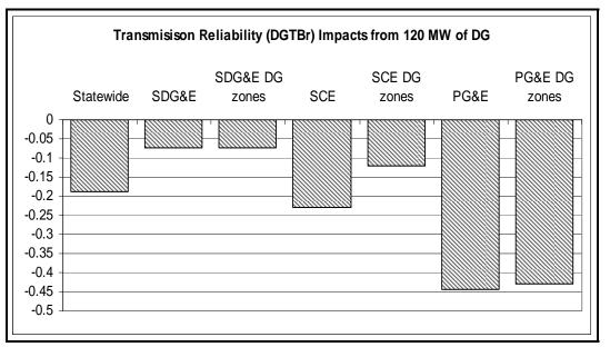
Figure B-9: Transmission Reliability Impacts from 120 MW of Self-Generation
