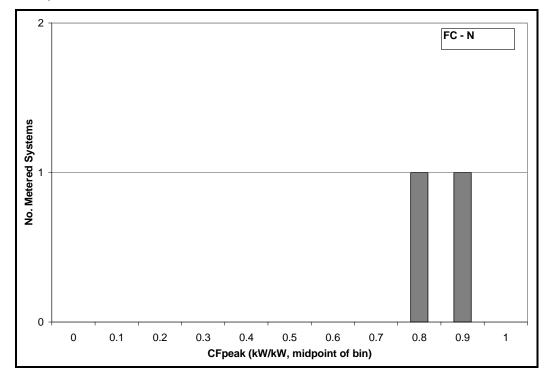
Figure D-23: Fuel Cell Measured Coincident Peak Output (Nonrenewable Fuel)
