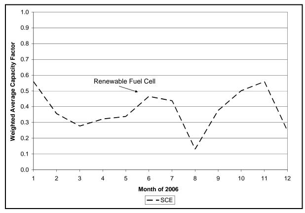
Figure A-18: Monthly Capacity Factors by PA
