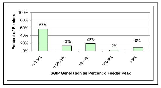
Figure B-35: Distribution of SGIP Generation as Percent of Feeder Peak - 2005
