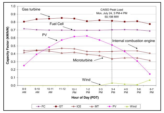
Figure 5-2: CAISO Peak Day Capacity Factors by Technology
