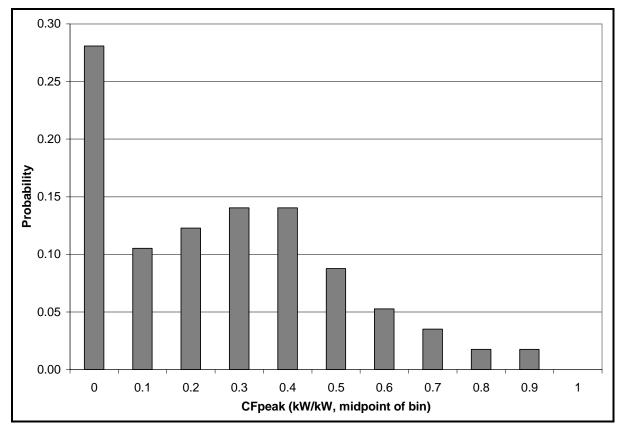
Figure D-3: CFpeak Distribution used in MCS for Renewable-Fueled Microturbines
