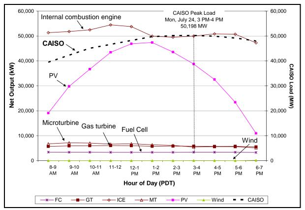
Figure 1-5: SGIP Project Impacts on 2006 System Peak Technology
