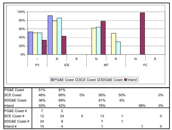
Figure B-26: Generation as a Percent of Operational Capacity by Climate Zone – 2005
