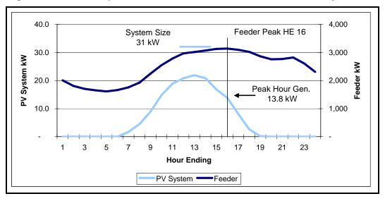
Figure B-10: Example Feeder Peak Hour Generation for PV system
