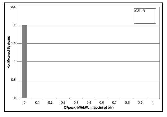
Figure D-29: IC Engine Measured Coincident Peak Output (Renewable Fuel)
