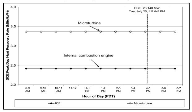
Figure 5-22: Heat Recovery Rate during SCE Peak Day
