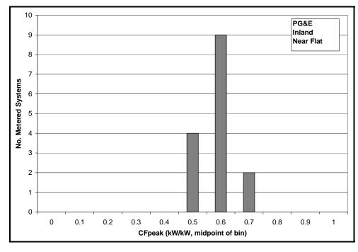
Figure D-5: PG&E PV Measured Coincident Peak Output (Inland, Near Flat)
