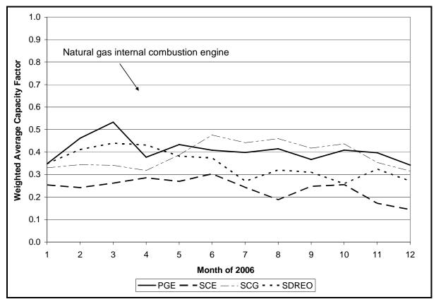
Figure A-33: Monthly Capacity Factors by Technology—Natural Gas ICE
