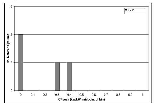
Figure D-35: Microturbine Measured Coincident Peak Output (Renewable Fuel)
