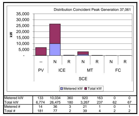
Figure B-18: Metered and Estimated Total Generation – SCE
