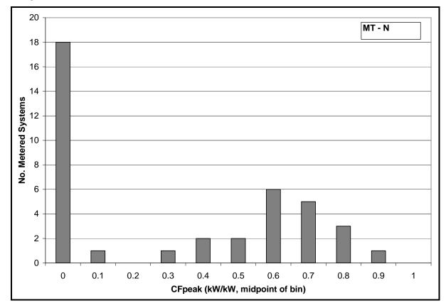
Figure D-1: Nonrenewable-Fueled Microturbine Measured Coincident Peak Output
