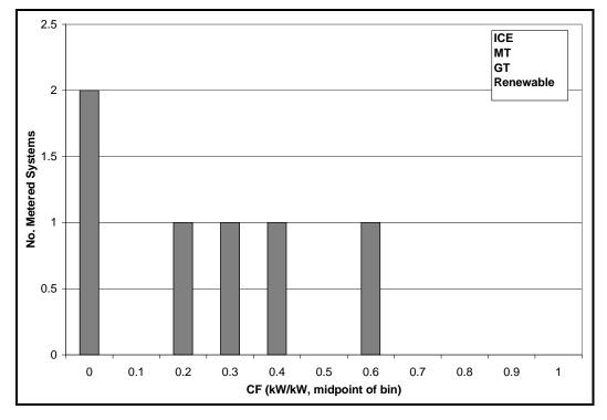
Figure D-47: Engine/Turbine (Renewable) Measured Electricity Production (Capacity Factor)
