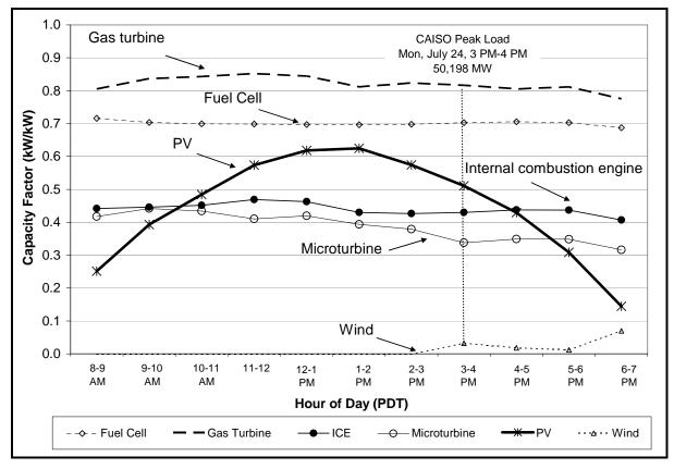
Figure A-6: CAISO Peak Day Capacity Factors by Technology
