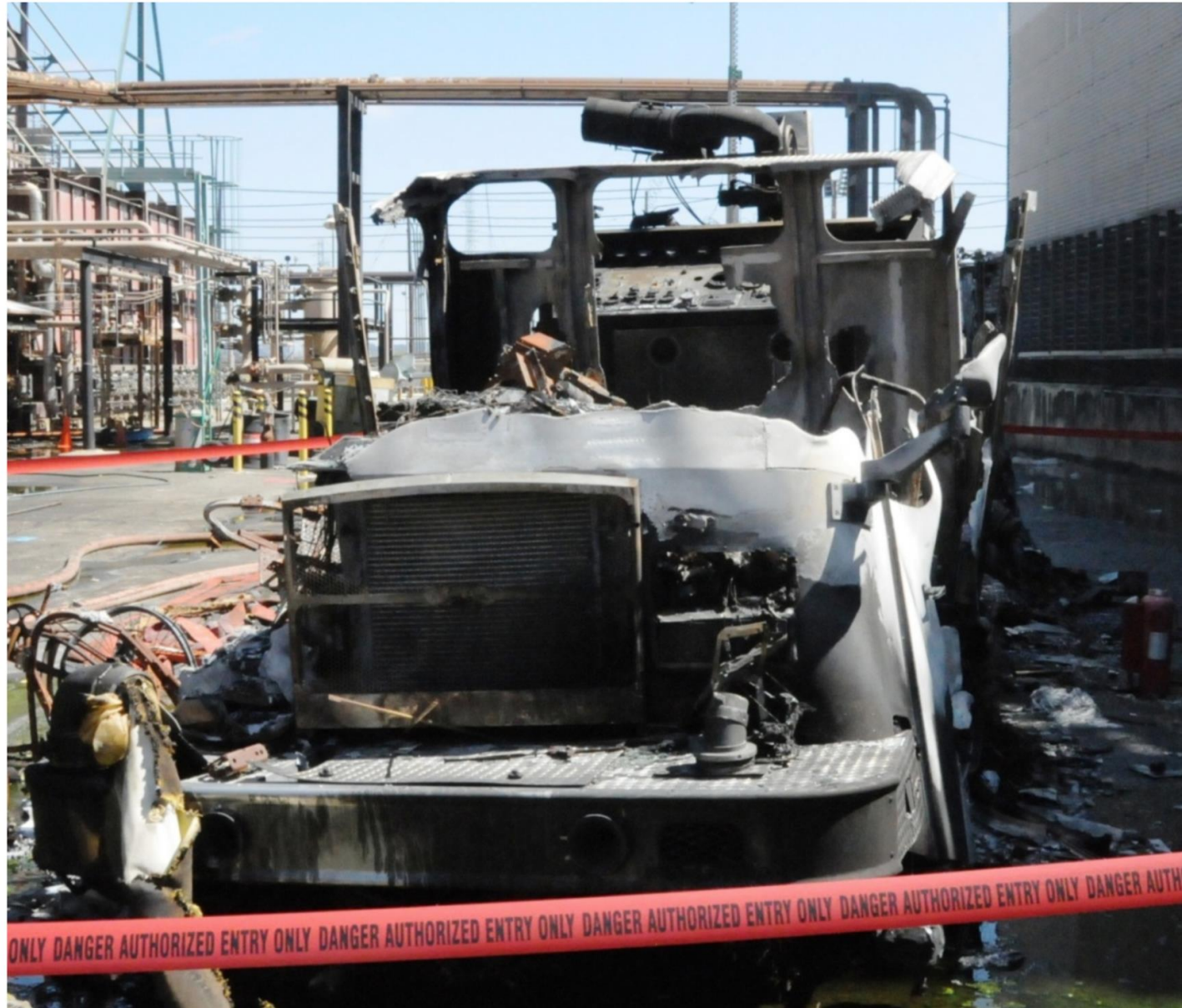
Figure 14. Photo of the burned remains of the fire truck that was consumed by the fire. A firefighter was in the cab when the light gas oil ignited. The fire truck was positioned in the cold zone approximately 65 feet from the leak location.
