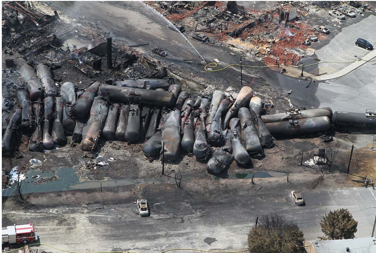
Destroyed tank cars Car type: USDOT Class DOT-111
